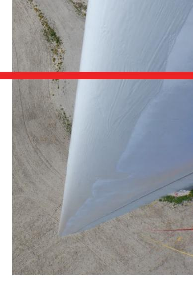
The image on the left shows one of the blades after being inspected by a drone 7 months in service. The products appears to be intact with no signs of wear, checking or peeling.
